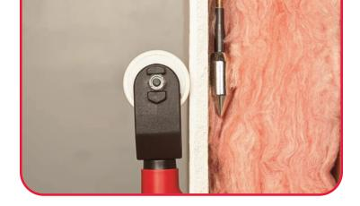
MAGNEPULL is designed for commercial or residential installations of cable, satellite TV, home theater, security and telecom wiring eliminating the problems associated with wire fishing.
